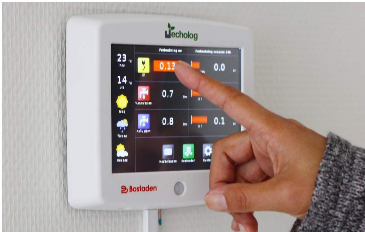
Figure 1C1. In all its new buildings Bostaden charges tenants individually for electricity, cold and hot water, visualizing their consumption (see above) on a display in the apartment.
