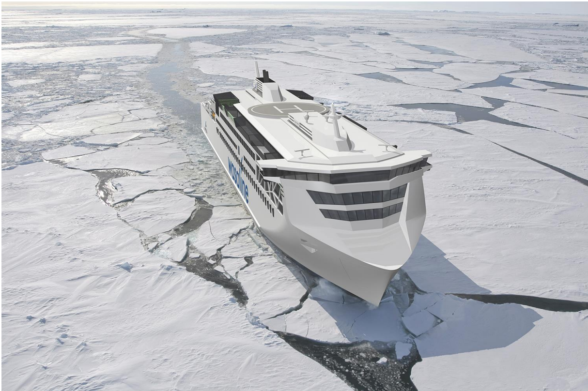
Figure 2C3. Artistic impression of new liquid natural gas ferry between Umeå and Vaasa, Finland as a part of the NLC corridor. The ferry will halve GHG emissions compared to today's values. LNG fuel will also help meet the standards of the EU sulphur directive (Directive 2012/33/EU). The ferry will be important for both goods and passenger transport between the two countries and further on.
